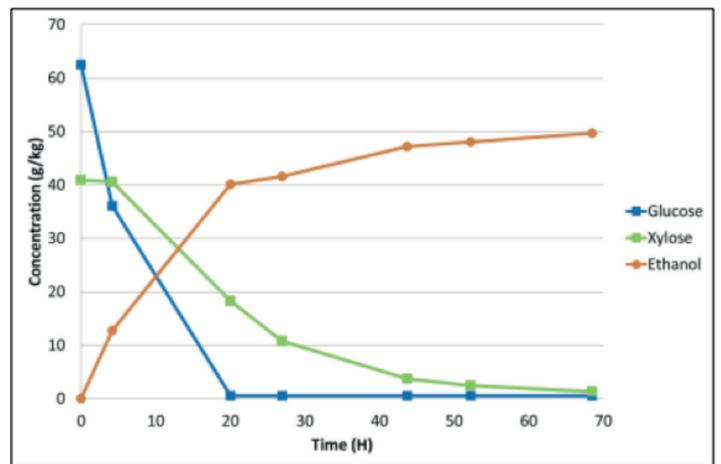
Fermentation results on Proesa technology – medium dry solids material – temperature: 32°C, pH: 5.5
