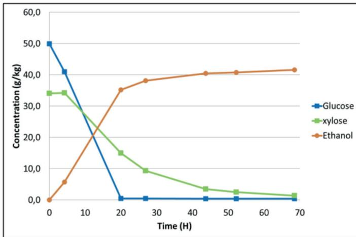
Fermentation results on Proesa technology – low dry solids material – temperature: 32°C, pH: 5.0
